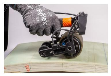
Krautkrämer RotoArray comPAct is suitable for ultrasonic NDT inspection of composite materials.
